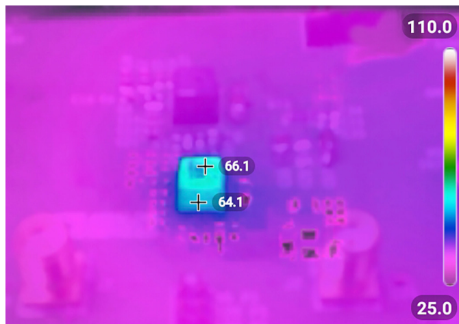
Figure 7. Thermal Image at 12V IN , 1V, 12A Output, No Airflow
