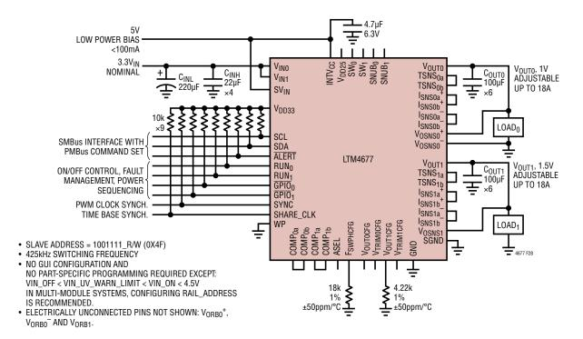
Figure 28. 18A, 1.0V and 1.5V Outputs Generated from 3.3V Power Input and Providing I<sup>2</sup>C/SMBus/PMBus Serial Interface
