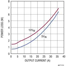
Figure 12. 1.2 $V_{OUT}$  Power Loss Curve
