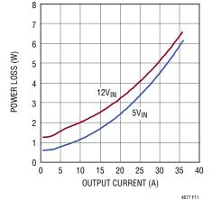
Figure 11. 0.9V<sub>OUT</sub> Power Loss Curve
