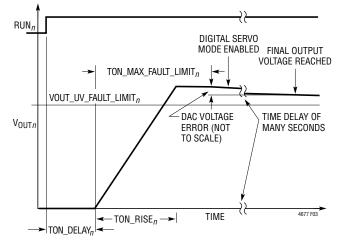
Figure 3. Timing Controlled  $V_{OUT}$  Rise
