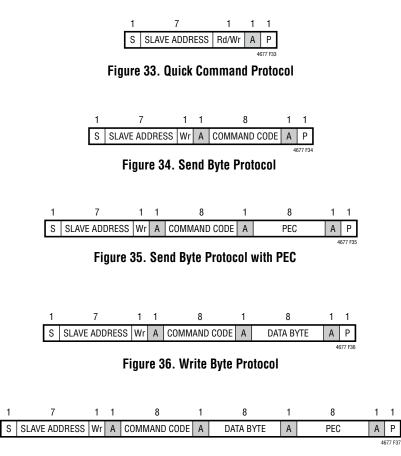
Figure 37. Write Byte Protocol with PEC
