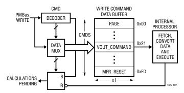
Figure 8. Write Command Data Processing
