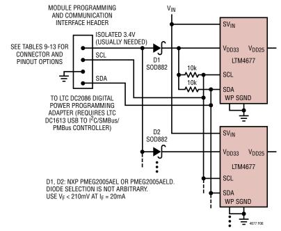
Figure 6. Circuit Suitable for Programming EEPROM/NVM of LTM4677 and Other ADI PSM Modules/ICs in Vast Systems, Even When  $V_{IN}$  Power is Absent, 0°C <  $T_J \le 85$ °C
