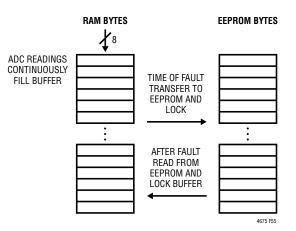
Figure 55. Fault Log Conceptual Diagram
