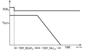
Figure 4. TOFF\_DELAY<sub>n</sub> and TOFF\_FALL<sub>n</sub>
