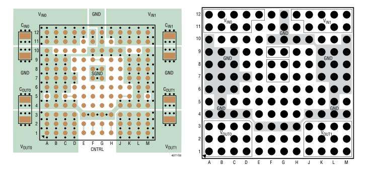
Figure 26. Recommended PCB Layout Package Top View, Universally Accommodates LTM4677, LTM4676A, and LTM4675 Modules
