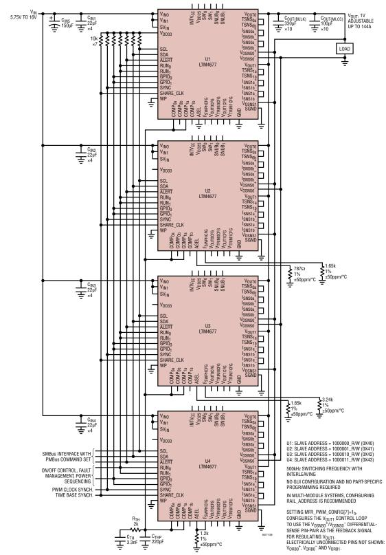
Figure 29. Four Paralleled LTM4677 Producing 1V<sub>OUT</sub> at Up to 144A. Integrated Power System Management Features Accessible Over 2-Wire I<sup>2</sup>C/SMBus/PMBus Serial Interface. For Evaluation and More Information, See Demo Boards DC2143
