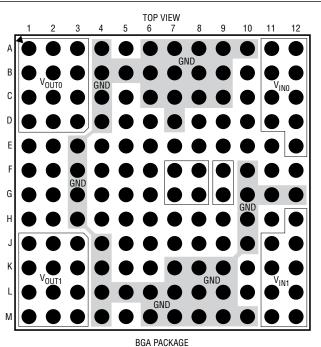
BGA PACKAGE 144-LEAD (16mm × 16mm × 5.01mm)
