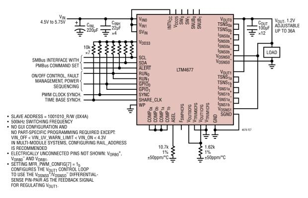
Figure 27. 36A, 1.2V Output DC/DC µModule Regulator with I<sup>2</sup>C/SMBus/PMBus Serial Interface
