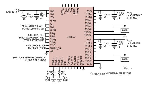
Test Circuit 1. LTM4677 ATE High V\_{IN} Operating Range Configuration, 5.75V  $\leq$  V\_{IN}  $\leq$  16V
