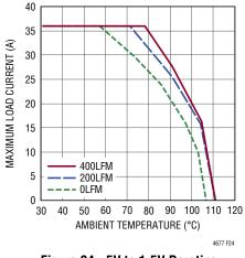
Figure 24. 5V to 1.5V Derating Curve, with Heat Sink
