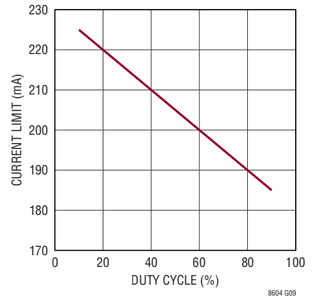
Top FET Current Limit vs Duty Cycle
