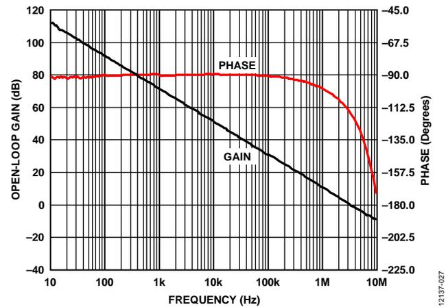
Figure 27. Open-Loop Gain and Phase vs. Frequency
