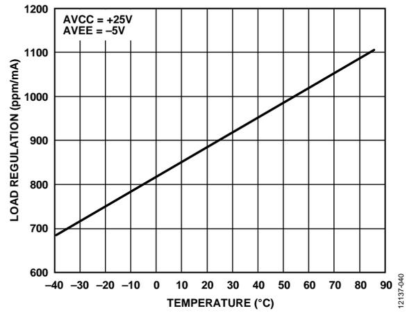
Figure 40. Source and Sink Load Regulation vs. Temperature
