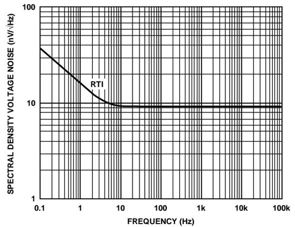
Figure 14. Spectral Density Voltage Noise, RTI vs. Frequency
