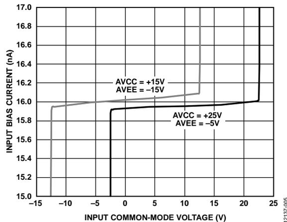
Figure 5. Input Bias Current vs. Input Common-Mode Voltage
