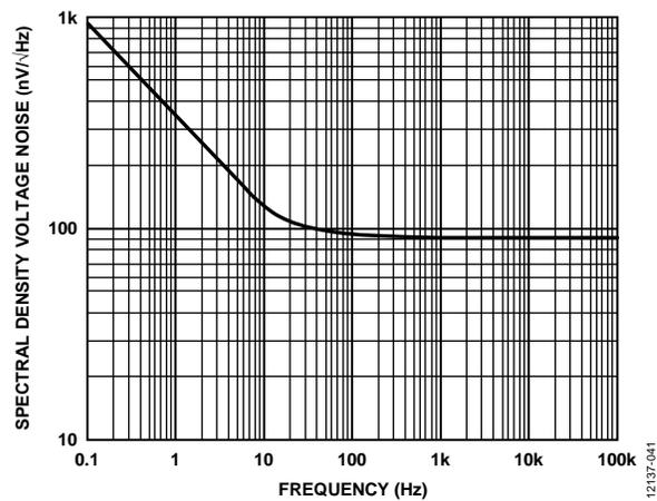
Figure 41. Spectral Density Voltage Noise vs. Frequency
