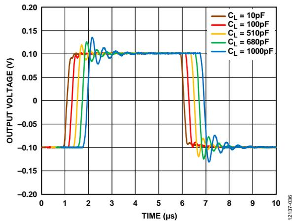
Figure 36. Small Signal Transient Response vs. Capacitive Load
