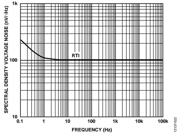
Figure 22. Spectral Density Voltage Noise, RTI vs. Frequency
